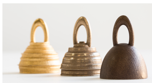
Figure 3 3D printed brass bells. Professor Stephen Barrass, 2017
